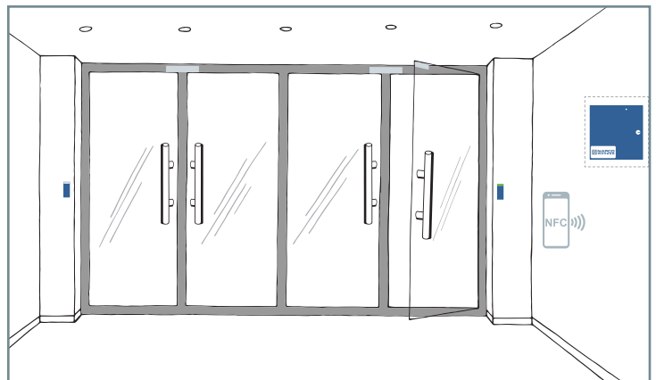
Making Any Grand Entrance Grander & More Convenient to Access with IDs in Phone Wallet (Similar to that shown on cover.) Here, 2 slim NFC mullion readers sit beside glass doors topped by mag locks, controlled by an NA-Series Panel, supporting NFC, biometrics, Prox, MiFare & Bluetooth
